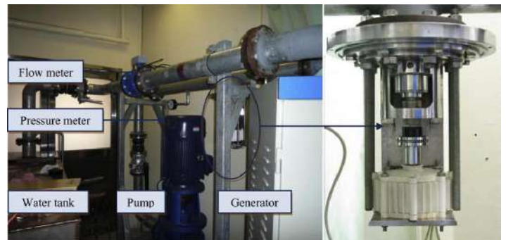
Fig.9 Whole testing rig of J. Chen et. al. (2013)
